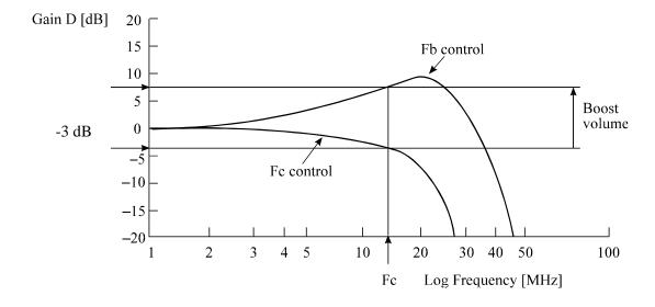
Figure 4.5 Frequency characteristic of programmable filter
